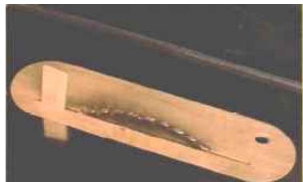
Simple but safe. A splitter is essential to any safe shop, but it doesn't have to cost a thing. Flip a zeroclearance insert end for end and raise the blade to elongate the slot. Fit a piece of hardwood tightly into the slot and then glue it in place.
