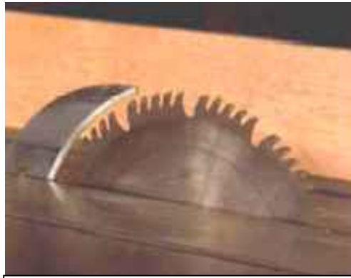
The best splitter closely hugs the back of the blade and can be left in place for all operations
