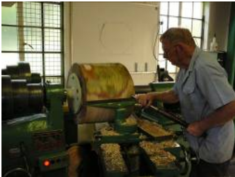
A 83 Kg Fever tree blank being rounded off. A sketch of the bowl envisaged is on the white board behind the lathe.
