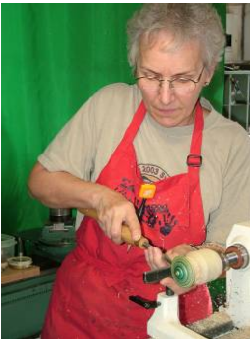
Turning a spinning top with a spindle gouge. Note the firm grip of the tool under the arm.
