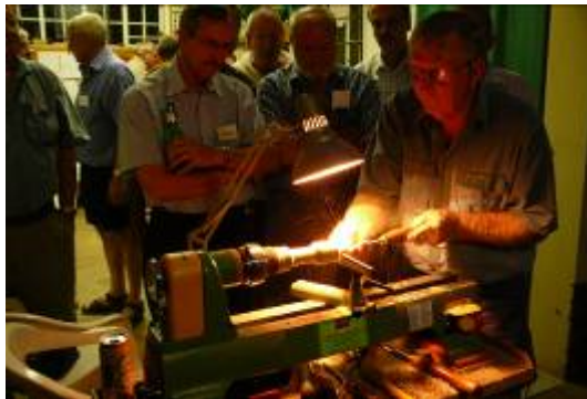
At Smit demonstrates the turning of a goblet, including a captive ring.
