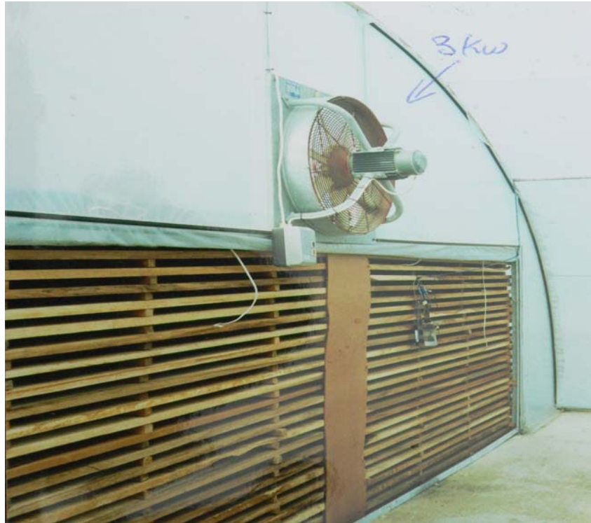
Fig. 2: Fan mounted in (transparent) fan wall above wood stacks
