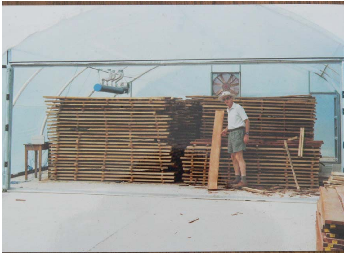
Fig. 3 Interior of a solar kiln during loading. The small blower (top left) and a feed back vent hole under table can be seen.
