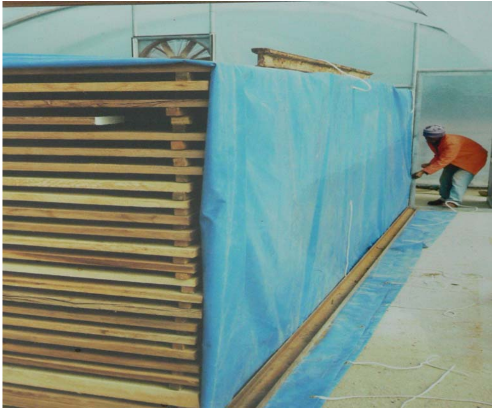
Fig. 4 Tarpaulin over stack with ends of stack open to allow airflow. Fan just visible above stack
